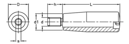
$$\begin{array}{ll} D & = 23 \\ d1 & = 19 \\ d \ 6g = M8 \\ h & = 17 \\ L & = 65 \\ s & = 6 \end{array}$$
